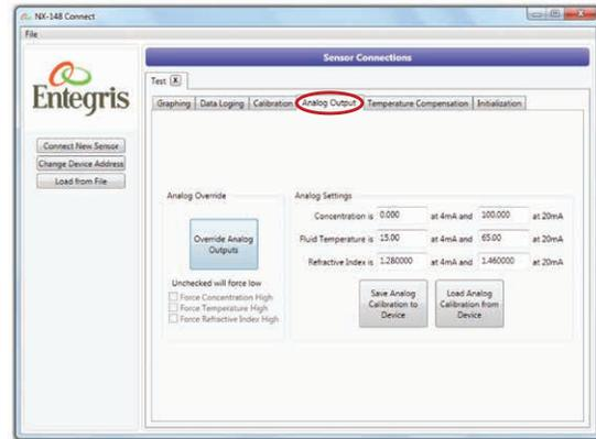
2. Configure the NX148 sensor's analog settings to match the user's 4–20 mA settings.
