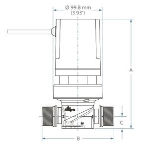
CV7 – CV8 Ranges (Flaretek ¾" and 1" Inlet /Outlet Type)
