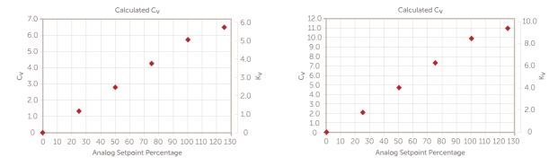
Graph data is representative and each valve needs to be characterized with the application to optimize performance.
